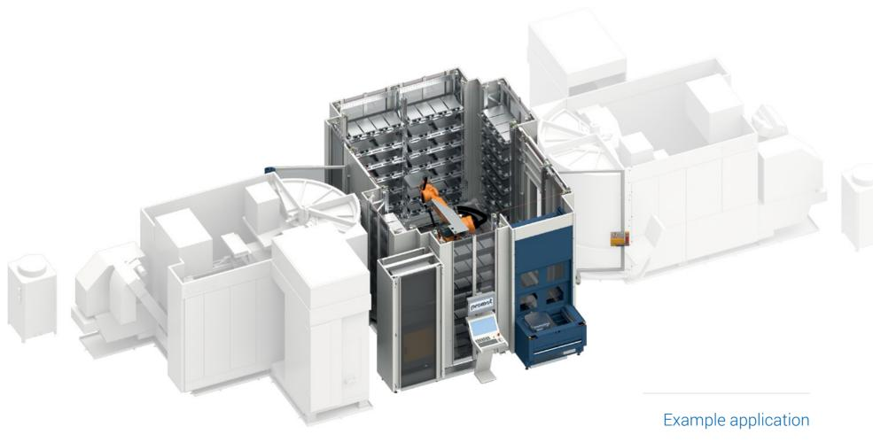
With our classic robot cell, a second machine can also be integrated afterwards.
